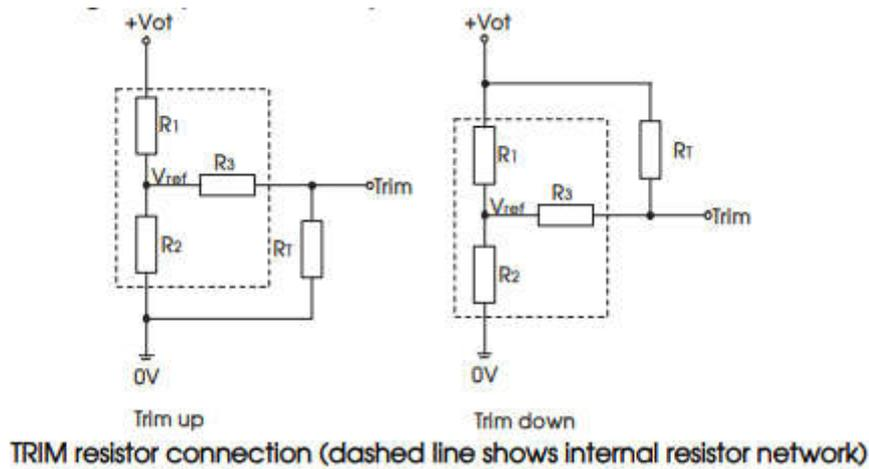
Diagram 4-6 Output Voltage Adjustment Schematic Diagram
