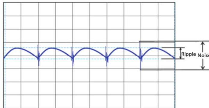
Diagram 4-4 Waveform of Ripple & Noise Test
