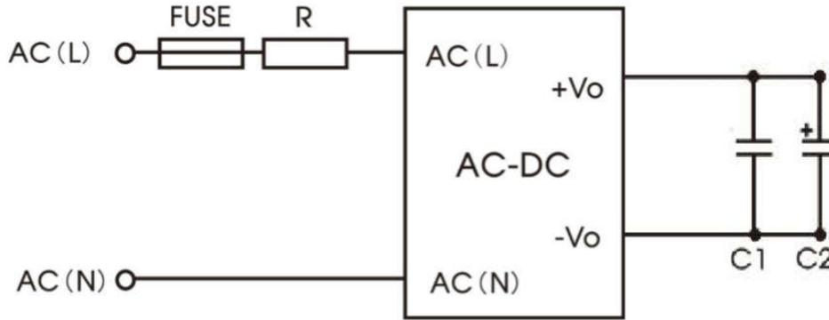
Diagram 3-1 EMC Solution-recommended Circuit
