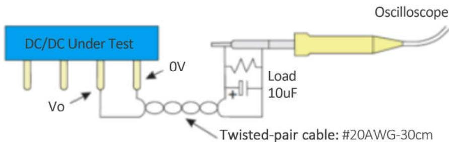
Diagram 4-2 Twisted-pair cable measuring method
