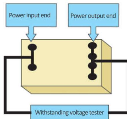
Diagram 4-5 Method of Withstand Test
