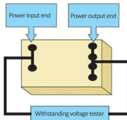
Diagram 4-5 Method of Withstand Test
