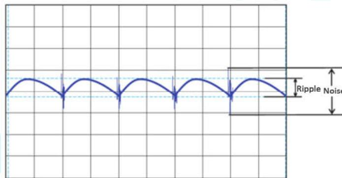
Diagram 4-4 Waveform of Ripple &amp; Noise Test
