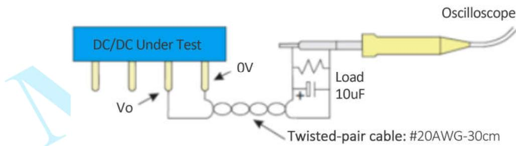
Diagram 4-2 Twisted-pair cable measuring method
