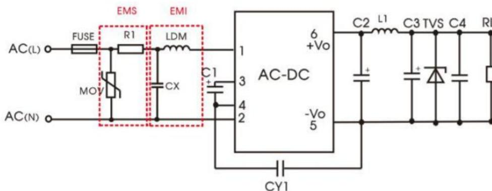
Figure 3-2 Typical application circuit of conventional LS series products (LO series products usually do not require peripheral circuits)
