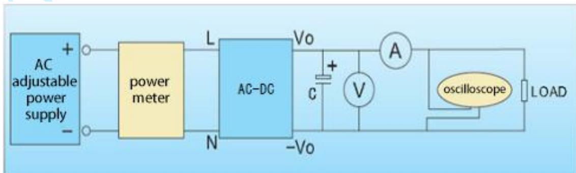
Figure 3-1 Circuit connection for Basic Test
