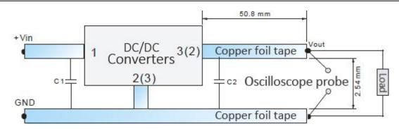
Diagram 2-3 Connection of dynamic load Test
