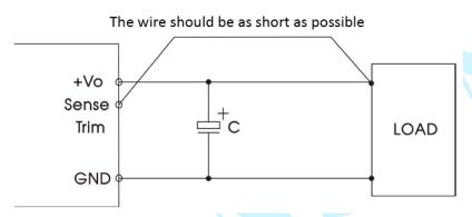
Diagram 3-9 Sense pin remote compensation application
