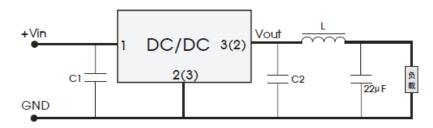
Diagram 3-5 Recommended circuit reducing ripple & noise
