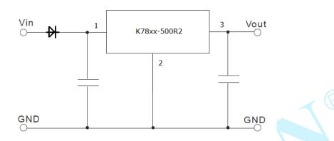
Diagram 3-4 Input reverse polarity protection circuit
