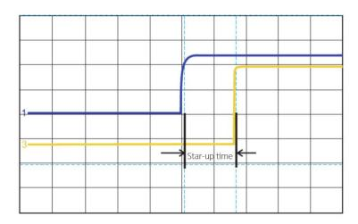
Diagram 2-6 Waveform of Start-up Time Test
