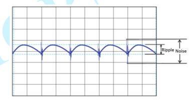
Diagram 2-2 Waveform of Ripple & Noise Test
