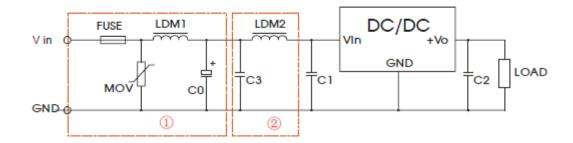
Diagram 3-6 EMC Solution-recommended Circuit
