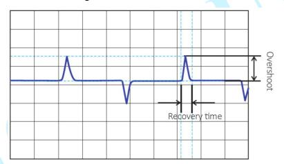
Diagram 2-4 Waveform of dynamic load Test
