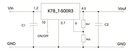
Diagram 3-4 Connection of output voltage trimming with an external resistor
