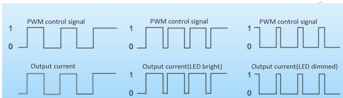
Diagram 3-5: PWM control signal and output current
