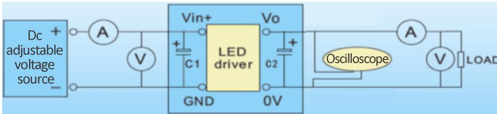
Diagram 2-1: LED Driver Test Method
