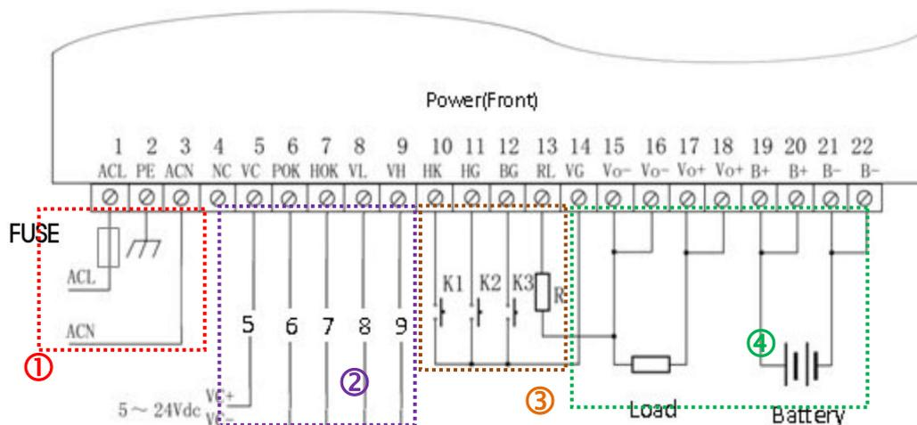
Figure 4-4: Typical Application Circuit of Battery Charging Power Supply
