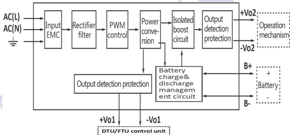
Figure 4-10: The Internal Functional Block Diagram for 220VDC Output Charging Power Supply
