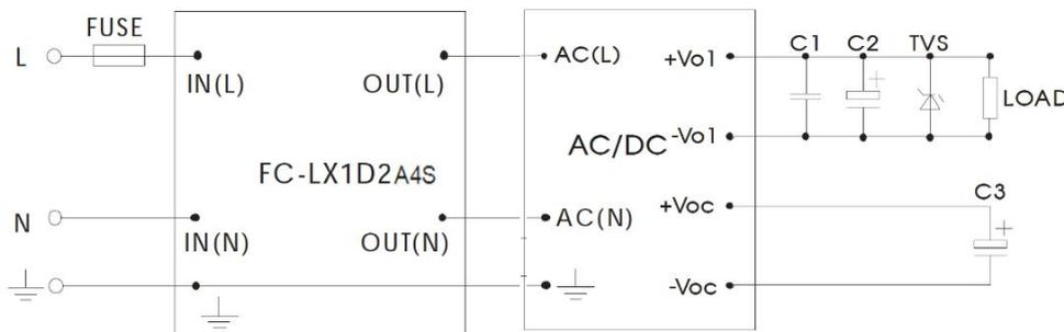
Figure 4-2: Typical Input EMC Filter Circuit
