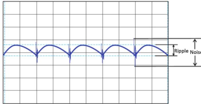
Figure 3-4: Ripple & Noise Test Waveform
