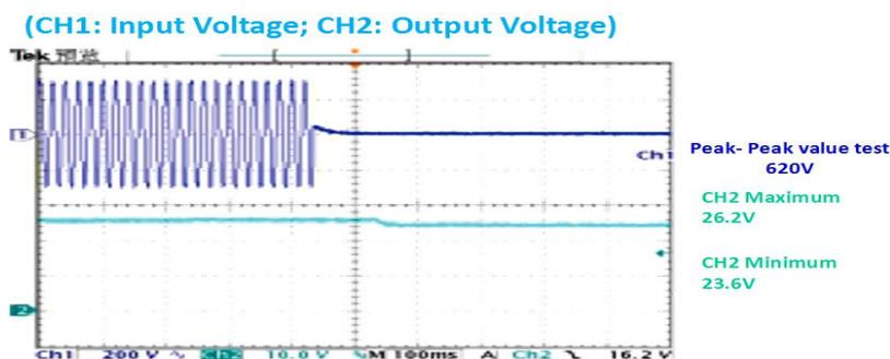
Figure 4-6: The Output UPS Voltage Waveform of Battery Charging Power Supply
