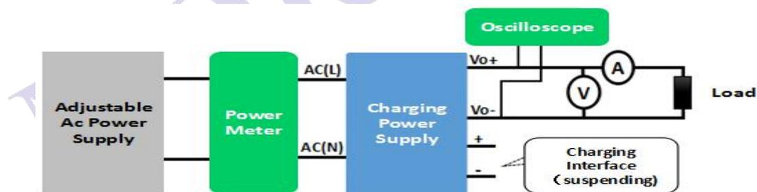
Figure 3-1: Basic Test Circuit Connection
