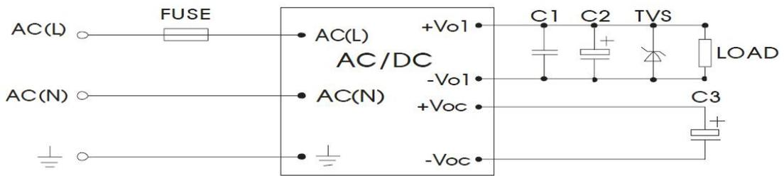
Figure 4-1: Typical Application Circuit of Capacitor Charging Power Supply
