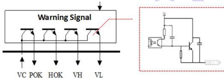
Figure 4-8: Operating Circuit Diagram of the Alarm Signal Port
