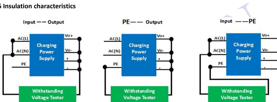
Figure 3-5: Withstand Voltage Test
