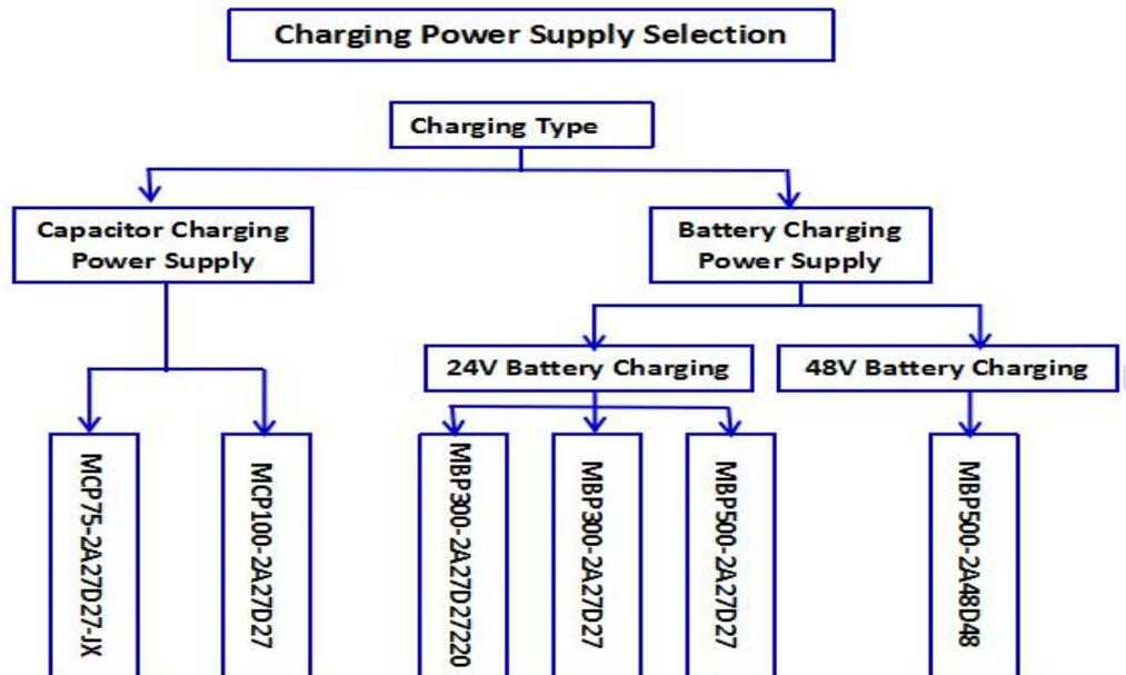
Figure 2-1: Selection Block Diagram
