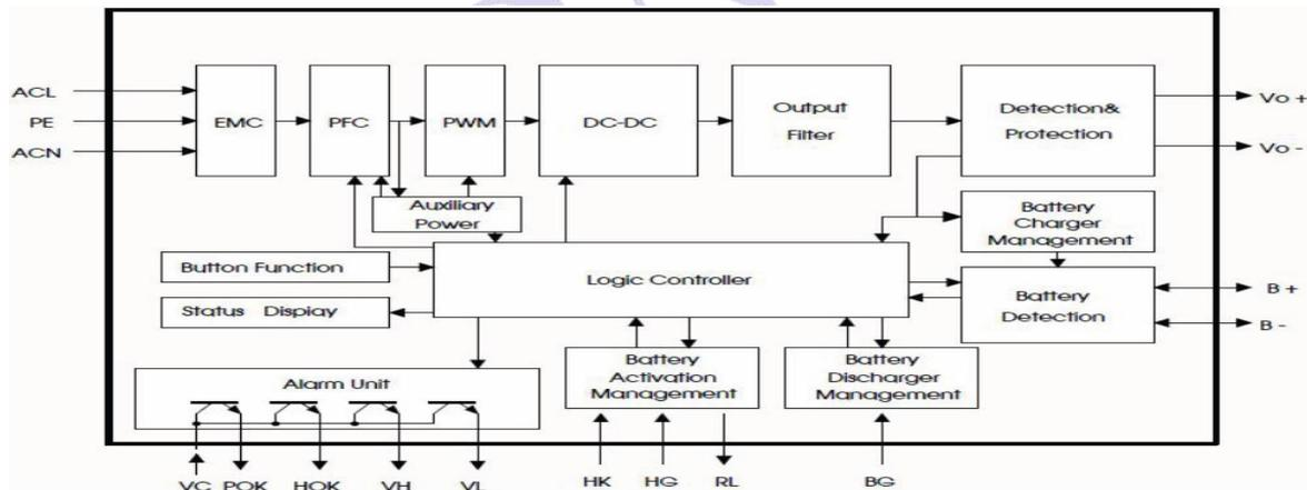
Figure 4-3: The Internal Functional Block Diagram of 27V/54V Output Charging Power Supply
